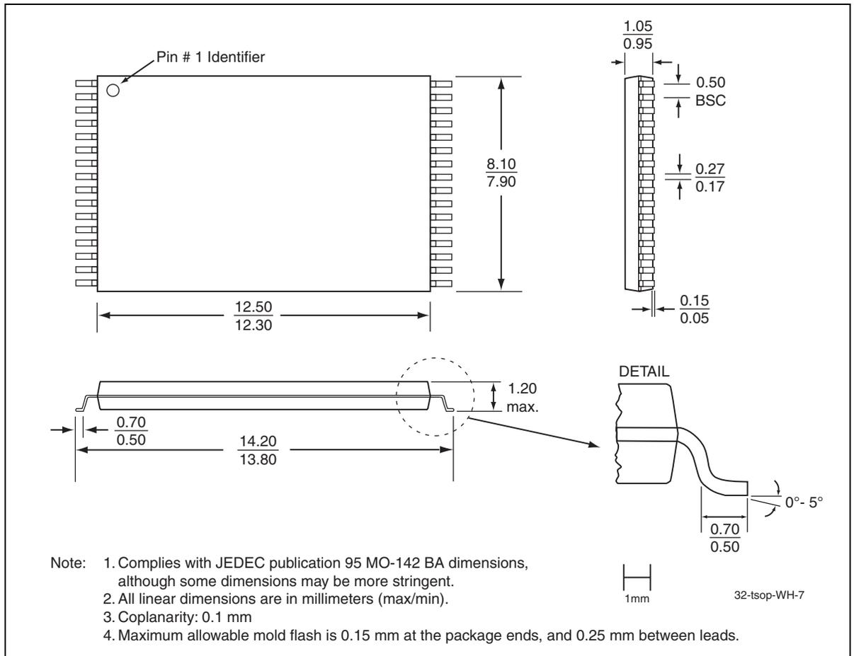
**Figure 21: 32-lead Thin Small Outline Package (TSOP) 8mm x 14mm**
