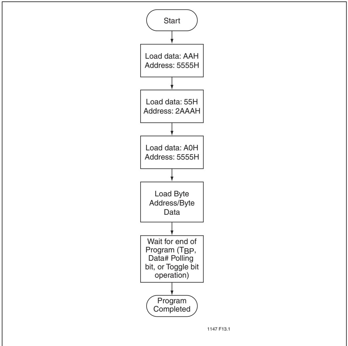
**Figure 16:**Byte-Program Algorithm
