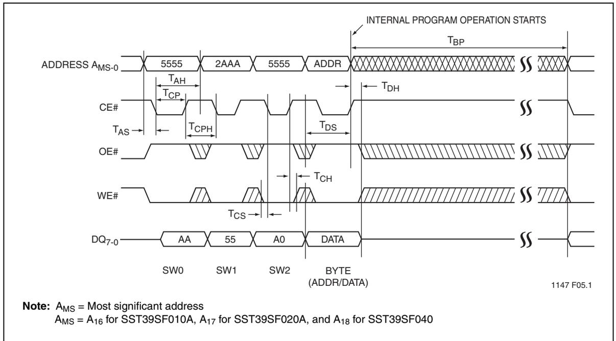
**Figure 7:** CE# Controlled Program Cycle Timing Diagram
