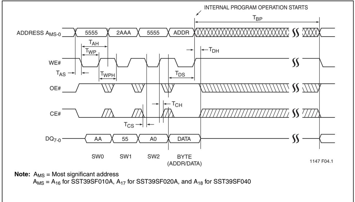
**Figure 6:** WE# Controlled Program Cycle Timing Diagram
