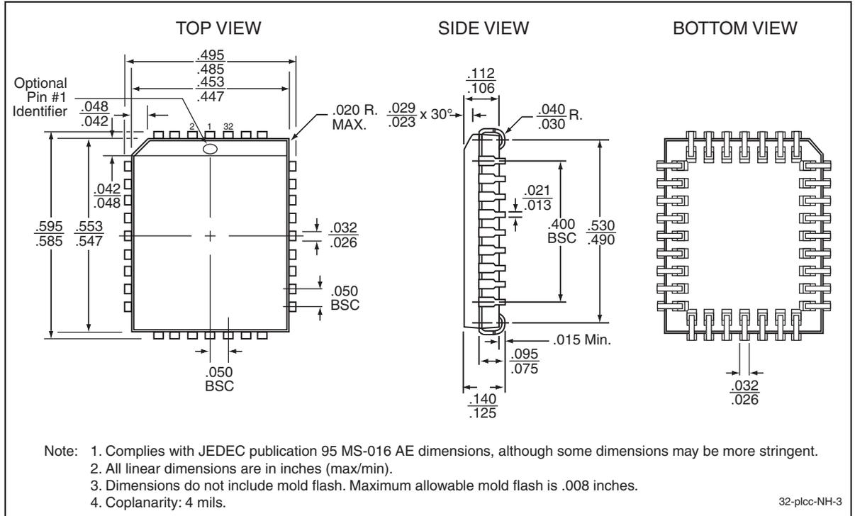
**Figure 20:32-lead Plastic Lead Chip Carrier (PLCC)**
