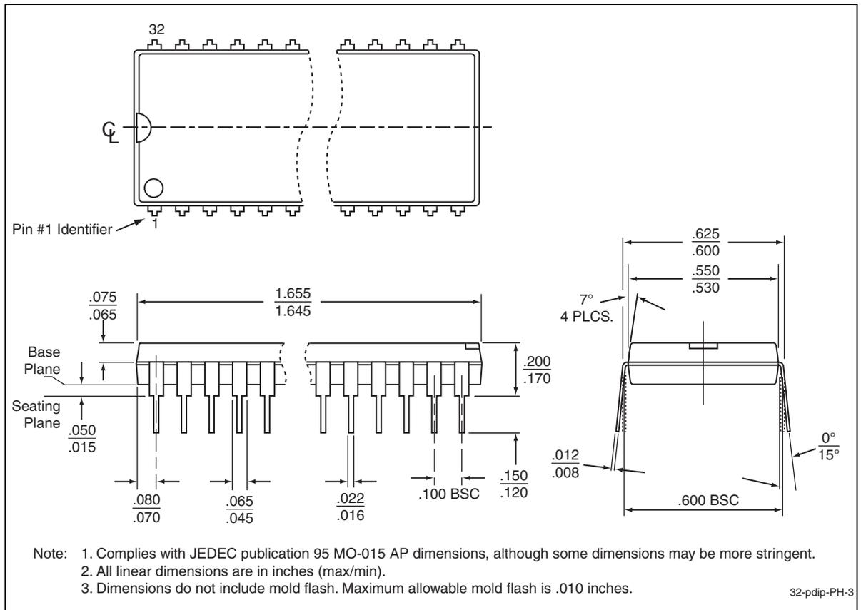
**Figure 22:** 32-pin Plastic Dual In-line Pins (PDIP)
