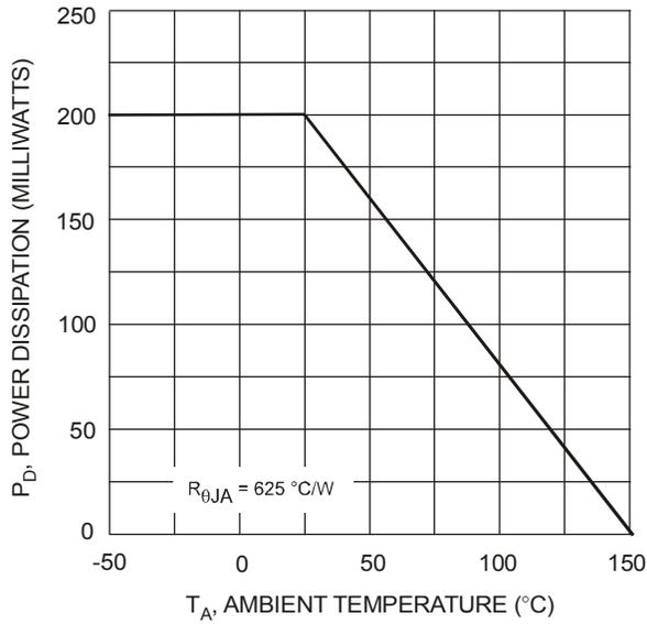
Fig. 1 Derating Curve
