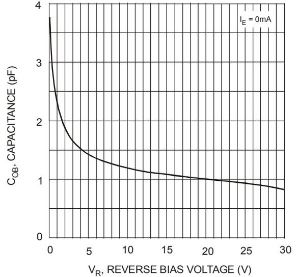
Fig. 4 Output Capacitance
