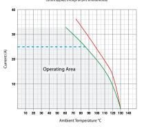
7000 Series Current vs. Temperature Characteristics
