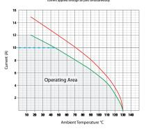
7000 Series Current vs. Temperature Characteristics
