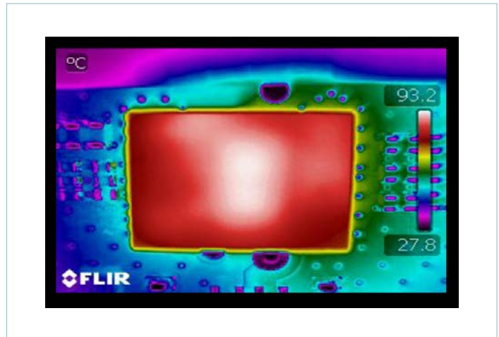
Figure 40 — Thermal image ( V_{IN} = 28V , I_{OUT} = 3.33A , CR, OLFM Evaluation PCB)
