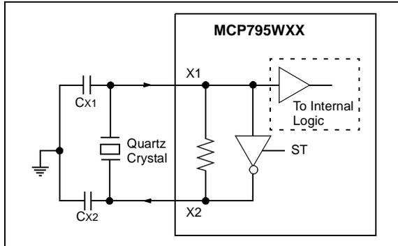
**Note 1:** The ST bit must be set to enable the crystal oscillator circuit.
