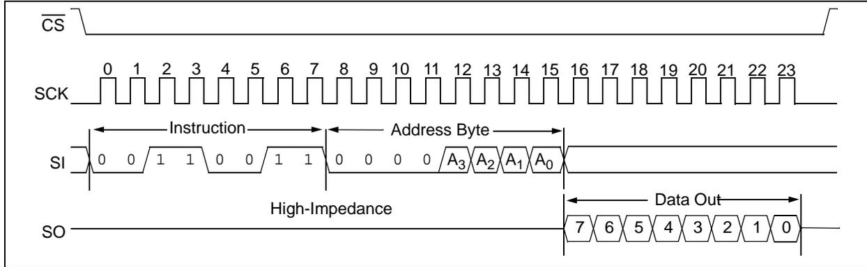
**FIGURE 6-12: PROTECTED EEPROM UNLOCK AND PAGE WRITE SEQUENCE**
