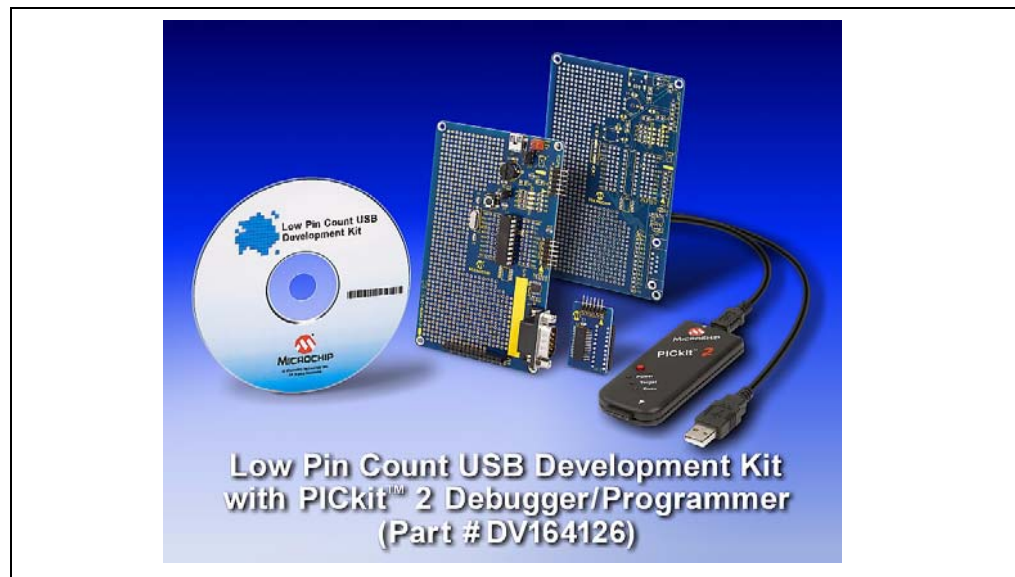
FIGURE 1-1: LOW PIN COUNT USB DEVELOPMENT KIT
