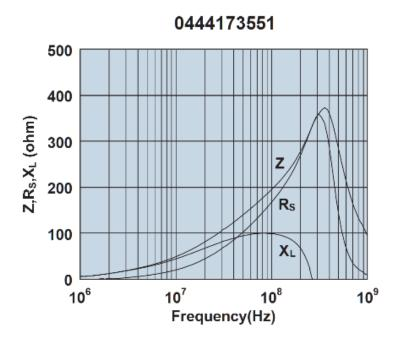
Impedance, reactance, and resistance vs. frequency.
