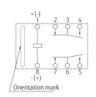
PC board mounting hole layout (BOTTOM VIEW)
