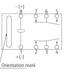
• PC board mounting pad layout (TOP VIEW)
