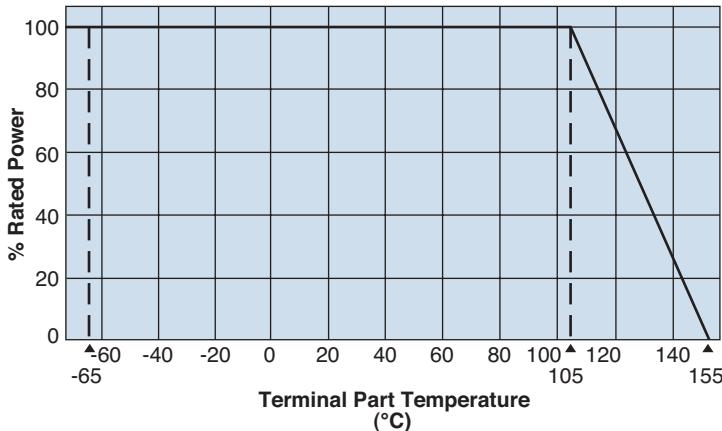
For resistors operated at a terminal part temperature of described for each size or above, a power rating shall be derated in accordance with the derating curve. Please refer to "Introduction of the derating curve based on the terminal part temperature" in the beginning of our catalog before use.
