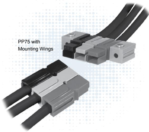
PP75 series Powerpole® housings can be used for wire-to-wire, wire-to-board, and wire-to-busbar applications. Wire sizes from #16 AWG (1.3 mm<sup>2</sup>) to #6 (13.3 mm<sup>2</sup>) offer power capabilities up to 120 amps per pole. Locking housings offer the capability to secure Powerpole® housings to each other and to mounting pads. Housings made from chemical resistant (CR) resin withstand industrial solvents better than standard housings.
