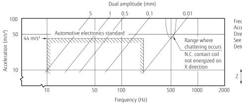
Frequency: 10 ~ 2000Hz Acceleration: 100m/s<sup>2</sup> max. Direction of vibration: See diagram below Detection level: Chatter >1ms
