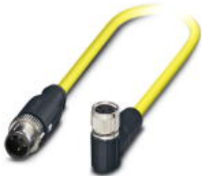
Sensor/actuator cable, 3-position, PVC, yellow, shielded, Plug straight M12 SPEEDCON, coding: A, on Socket angled M8, cable length: 0.5 m
