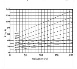
FIGURE 23-27: TYPICAL IDD vs. FREQUENCY (XT MODE, 25°C)
