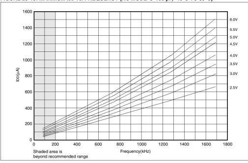
FIGURE 23-16: TYPICAL IDD vs. FREQUENCY (RC MODE @ 300 pF, 25°C)
