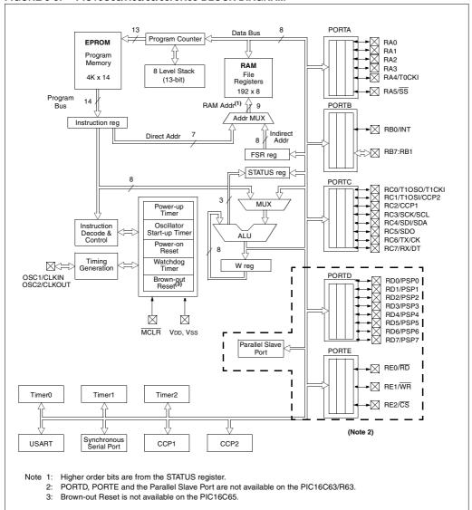
FIGURE 3-3: PIC16C63/R63/65/65A/R65 BLOCK DIAGRAM
