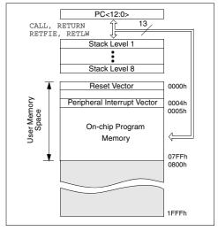
FIGURE 4-3: PIC16C63/R63/65/65A/R65 PROGRAM MEMORY MAP AND STACK
