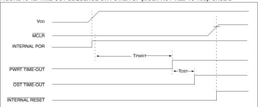
FIGURE 13-13: TIME-OUT SEQUENCE ON POWER-UP (MCLR TIED TO VDD)
