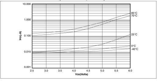
FIGURE 23-3: TYPICAL IPD vs. VDD @ 25°C (WDT ENABLED, RC MODE)
