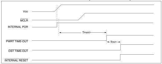
FIGURE 13-12: TIME-OUT SEQUENCE ON POWER-UP (MCLR NOT TIED TO VDD): CASE 2
