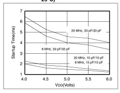
FIGURE 23-24: TYPICAL XTAL STARTUP TIME vs. VDD (XT MODE, 25°C)
