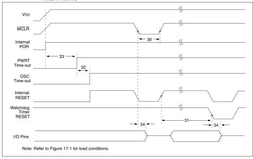
TABLE 17-4: RESET, WATCHDOG TIMER, OSCILLATOR START-UP TIMER AND POWER-UP TIMER REQUIREMENTS
