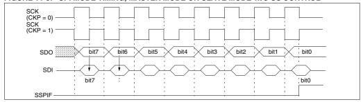
FIGURE 11-6: SPI MODE TIMING, SLAVE MODE WITH SS CONTROL
