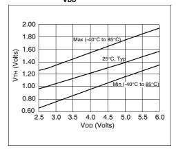
FIGURE 16-10: VIH, VIL OF MCLR, TOCKI AND OSC1 (IN RC MODE) vs. VDD
