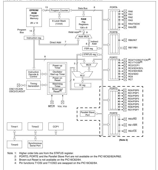
FIGURE 3-2: PIC16C62/62A/R62/64/64A/R64 BLOCK DIAGRAM
