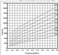
FIGURE 23-29: TYPICAL IDD vs. FREQUENCY (HS MODE, 25°C)
