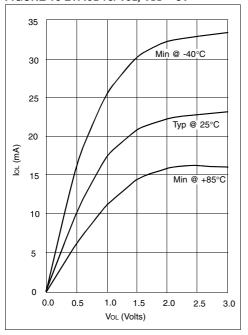
FIGURE 16-22: IOL VS. VOL, VDD = 5V
