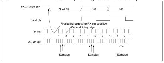
FIGURE 12-5: RX PIN SAMPLING SCHEME (BRGH = 1) (PIC16C63/R63/65/65A/R65)
