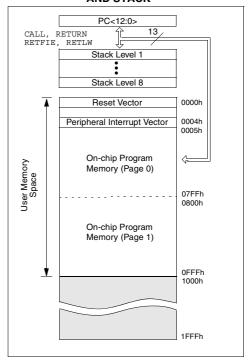
FIGURE 4-4: PIC16C66/67 PROGRAM MEMORY MAP AND STACK
