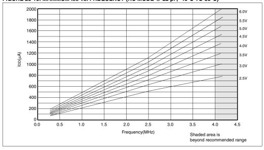
FIGURE 23-14: TYPICAL IDD vs. FREQUENCY (RC MODE @ 100 pF, 25°C)
