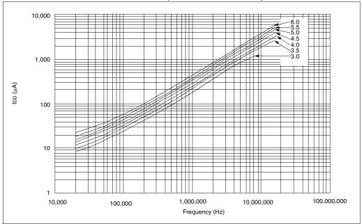
FIGURE 16-13: MAXIMUM IDD vs. FREQUENCY (EXTERNAL CLOCK, -40° TO +85°C)
