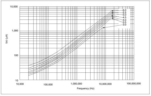
FIGURE 16-14: MAXIMUM IDD vs. FREQUENCY (EXTERNAL CLOCK, -55° TO +125°C)
