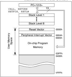
FIGURE 4-2: PIC16C62/62A/R62/64A/64A/ R64 PROGRAM MEMORY MAP AND STACK
