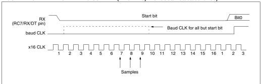
FIGURE 12-4: RX PIN SAMPLING SCHEME (BRGH = 1) (PIC16C63/R63/65/65A/R65)
