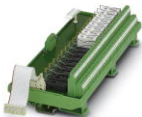
VARIOFACE output extension module, with plug-in bases for 16 miniature relays, with 2 PDTs each (without relays), for 24 V DC
