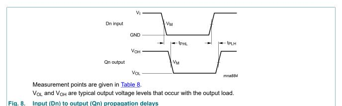
Input (Dn) to output (Qn) propagation delays
