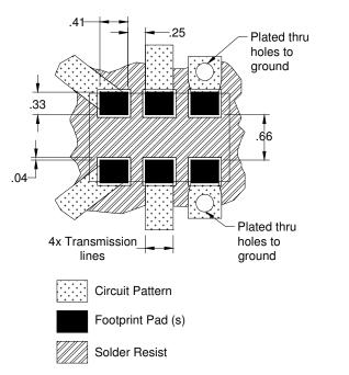
Dimensions are in Millimeters Mounting Footprint
