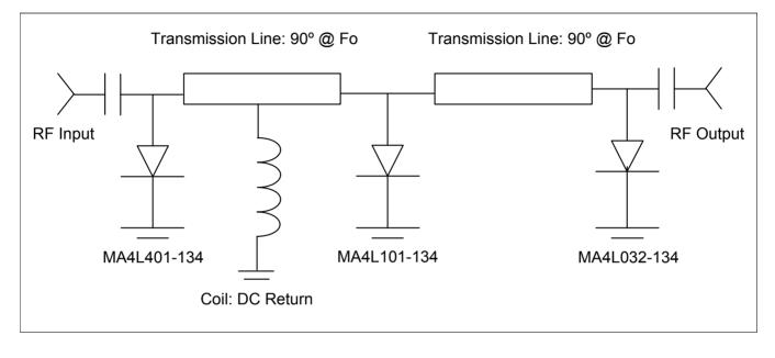
Typical 50 dBm Peak Power, 1 µs P.W., 0.1% Duty Cycle, 20 dBm Flat Leakage Limiter Circuit
