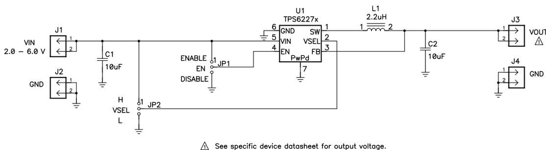
Figure 11. TPS6227XEVM-306 Schematic
