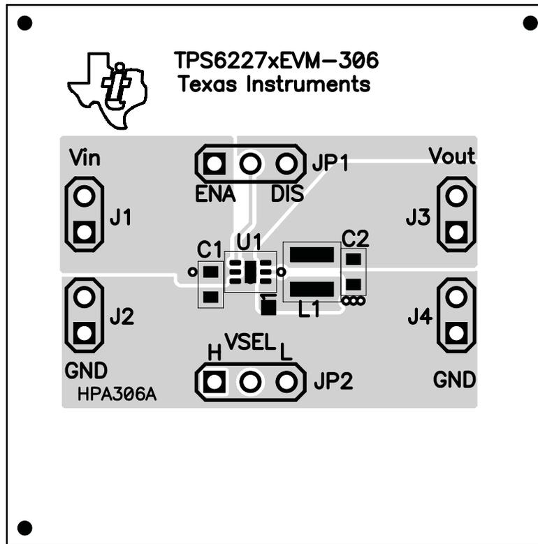
Figure 8. Assembly Layer
