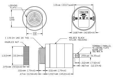
NOTE A: TERMINALS-.032 BRASS TIN PLATED, TAPPED FOR #6-32 SCREW. TWO #6-32 NICKEL PLATED BRASS SCREWS INCLUDED. WILL ACCEPT 1/4' QUICK CONNECT. NOTE B: MOUNTING- REMOVE BLACK PLASTIC NUT AND INSERT THREADED FRONT THROUGH 125' HOLE PUNCHED IN PANEL, IF DEKENTATION IS NEEDED, NOTE LOCKING FLATS ON DRAWING. SCREW NUT BACK ON. DO NOT DVERTIGHTEN.
