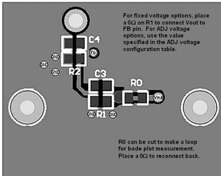
Figure 8. Bottom Layer (SOT23-5 and 5-bump DSBGA)
