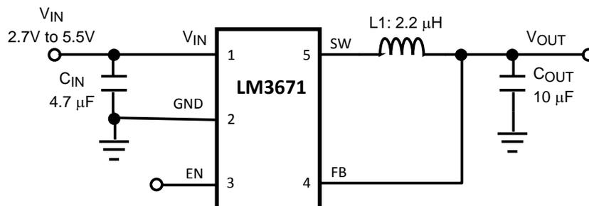
**Figure 1. Fixed Output Voltage — Typical Application Circuit**
