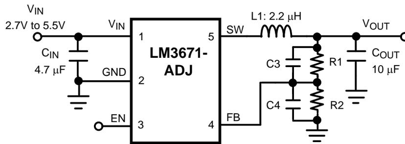
**Figure 2. Adjustable Output Voltage — Typical Application Circuit**
