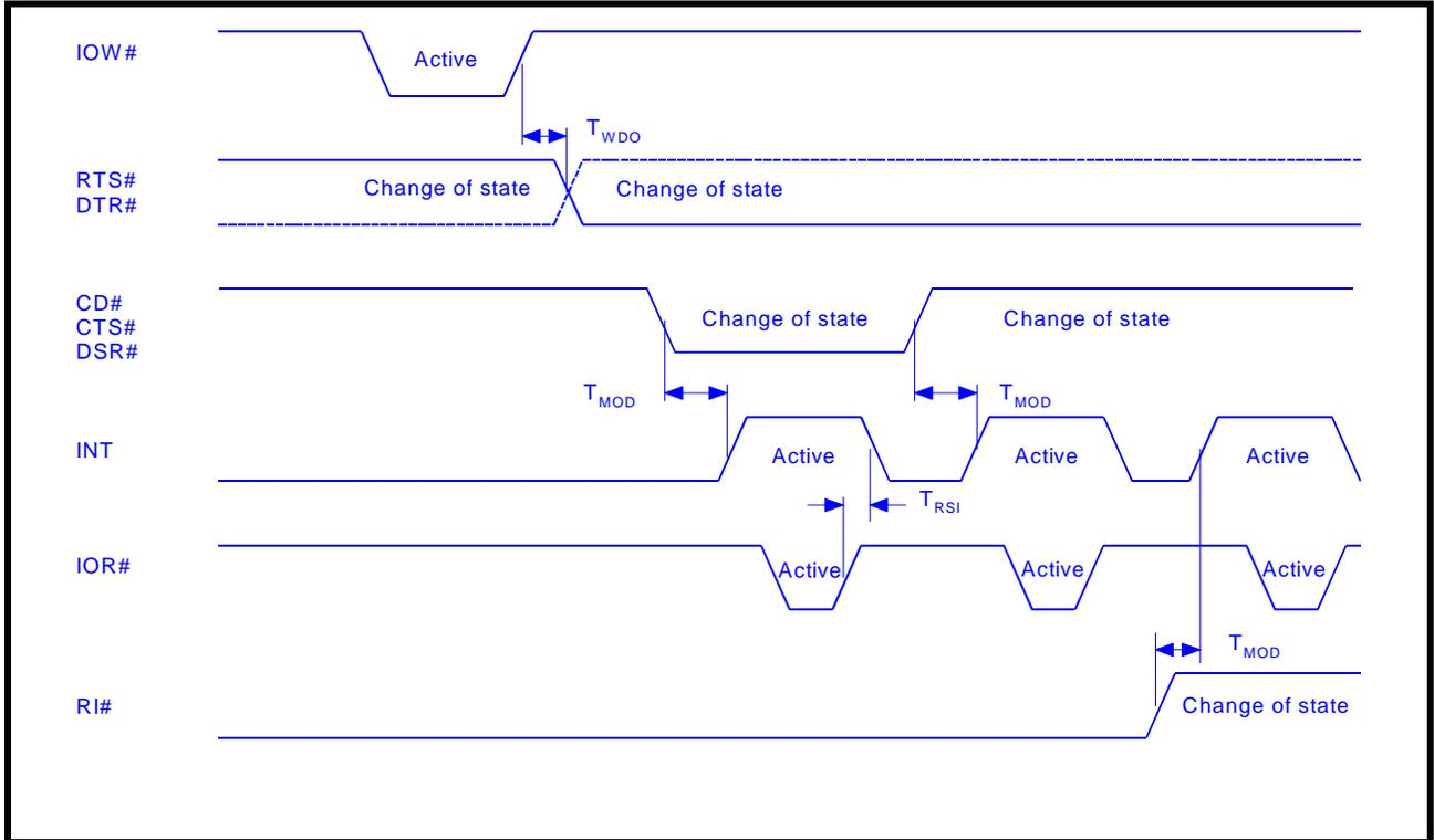
FIGURE 19. RECEIVE INTERRUPT TIMING [NON-FIFO MODE]
