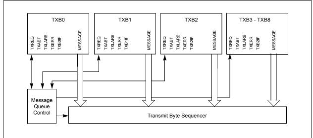
FIGURE 23-2: TRANSMIT BUFFERS
