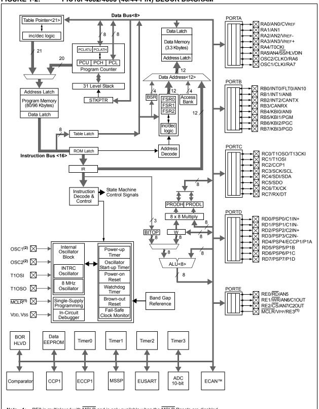
FIGURE 1-2: PIC18F4682/4685 (40/44-PIN) BLOCK DIAGRAM
