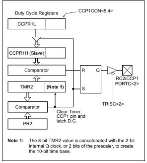
A PWM output (Figure 15-4) has a time base (period) and a time that the output stays high (duty cycle). The frequency of the PWM is the inverse of the period (1/ period).
