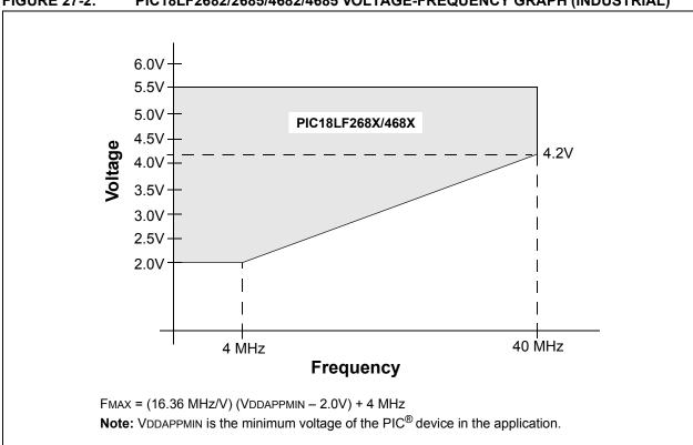
FIGURE 27-2: PIC18LF2682/2685/4682/4685 VOLTAGE-FREQUENCY GRAPH (INDUSTRIAL)
