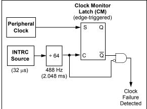
Clock failure is tested for on the falling edge of the sample clock. If a sample clock falling edge occurs while CM is still set, a clock failure has been detected (Figure 24-4). This causes the following:
