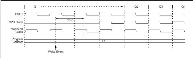
Note: The Timer1 oscillator should already be running prior to entering SEC\_IDLE mode. If the T1OSCEN bit is not set when the SLEEP instruction is executed, the SLEEP instruction will be ignored and entry to SEC\_IDLE mode will not occur. If the Timer1 oscillator is enabled but not yet running, peripheral clocks will be delayed until the oscillator has started. In such situations, initial oscillator operation is far from stable and unpredictable operation may result.
