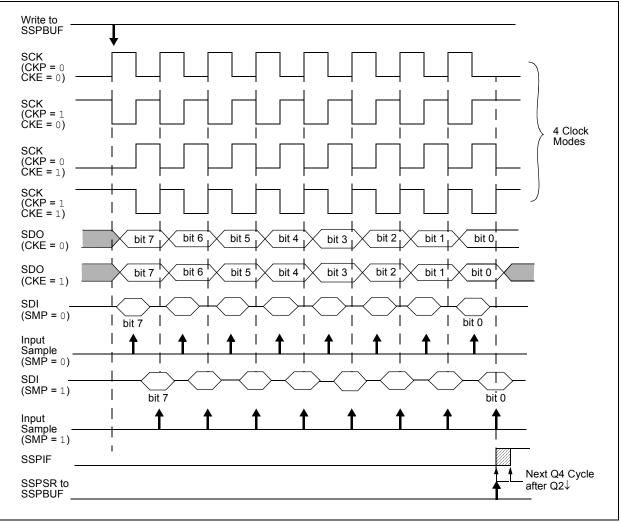
FIGURE 17-3: SPI MODE WAVEFORM (MASTER MODE)
