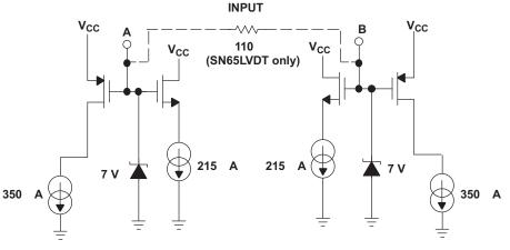
Figure 38. Receiver Equivalent Schematic
