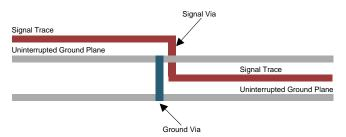
Figure 57. Ground Via Location (Side View)
