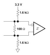
Figure 36. External Failsafe Circuit
