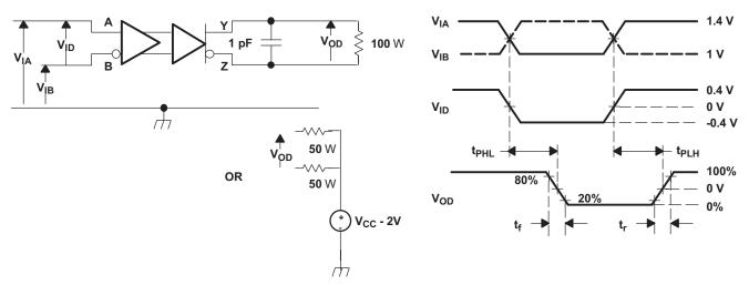
NOTE: All input pulses are supplied by a generator having the following characteristics: t<sub>r</sub> or t<sub>f</sub> ≤ 0.25 ns, pulse repetition rate (PRR) = 50 Mpps, pulse width = 10 ± 0.2 ns. C<sub>L</sub> includes instrumentation and fixture capacitance within 0.06 mm of the device under test. Measurement equipment provides a bandwidth of 5 GHz minimum.
