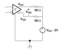
Figure 39. Typical Termination for LVPECL Output Driver (SN65LVDx101)
