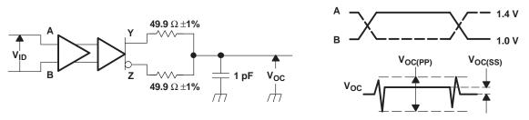
NOTE: All input pulses are supplied by a generator having the following characteristics: t<sub>r</sub> or t<sub>f</sub> ≤ 0.25 ns, pulse repetition rate (PRR) = 0.5 Mpps, pulse width = 500 ± 10 ns. C<sub>L</sub> includes instrumentation and fixture capacitance within 0.06 mm of the device under test. The measurement of V<sub>OC(PP)</sub> is made on test equipment with a –3 dB bandwidth of at least 300 MHz.
