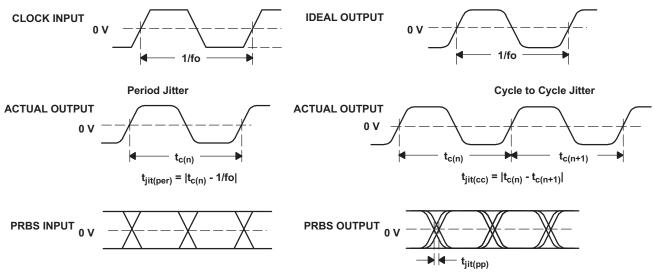
Figure 34. Driver Jitter Measurement Waveforms
