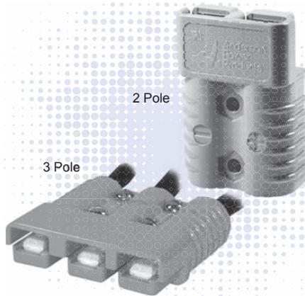
Wires sizes from #10 (5.3 mm<sup>2</sup>) to 1/0 (50 mm<sup>2</sup>) fit in the second to largest connector in the SB® series. The 3 pole SB®175 adds an additional position for power or grounding. All Multipole wire connector housings are genderless and mate to themselves minimizing inventory and assembly complexity.
