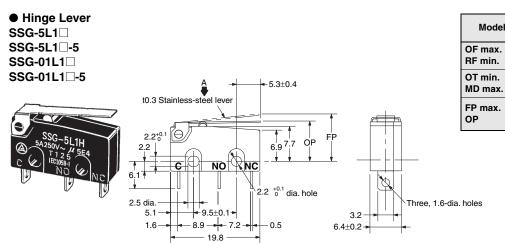
Note: Also available are models with a hinge lever length of 26.1 mm under the following model numbers; SSG-01L14□, SSG-5L14□, SSG-01L14□-5, and SSG-5L14□-5. Consult your OMRON sales representative for these models.
