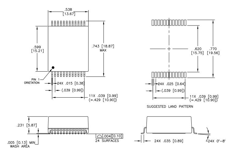
DIMENSIONS ARE IN INCHES [MILLIMETERS] WITH THE FOLLOWING TOLERANCES: [MILLIMETERS] ARE FOR REFERENCE ONLY.  $.XX = \pm .02 \qquad [\pm 0.5] \\ .XXX = \pm .010 \ [\pm 0.25]$
