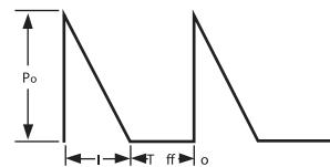
The Pulse Waveform, if other than square wave, must first be converted to an approximate square wave as shown below.
