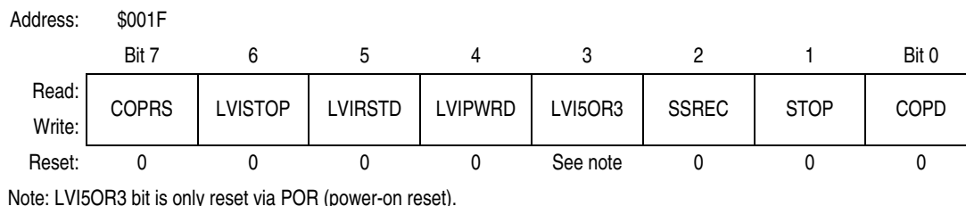
Figure 5-2. Configuration Register 1 (CONFIG1)
