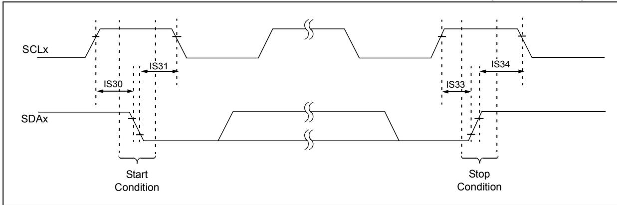
**TABLE 28-32: I<sup>2</sup>C™ BUS START/STOP BIT TIMING REQUIREMENTS (SLAVE MODE)**
