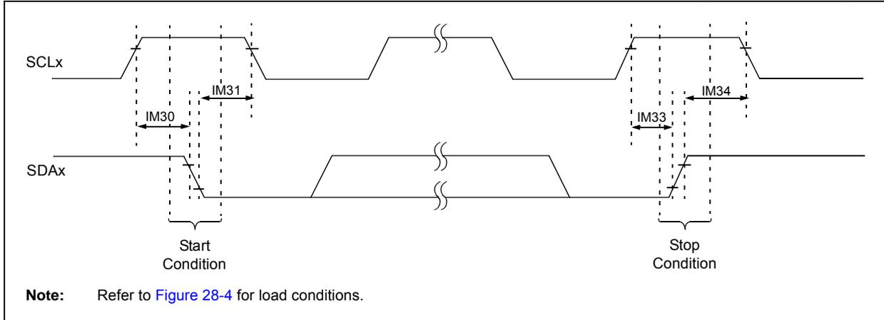
**TABLE 28-30: I<sup>2</sup>C™ BUS START/STOP BIT TIMING REQUIREMENTS (MASTER MODE)**
