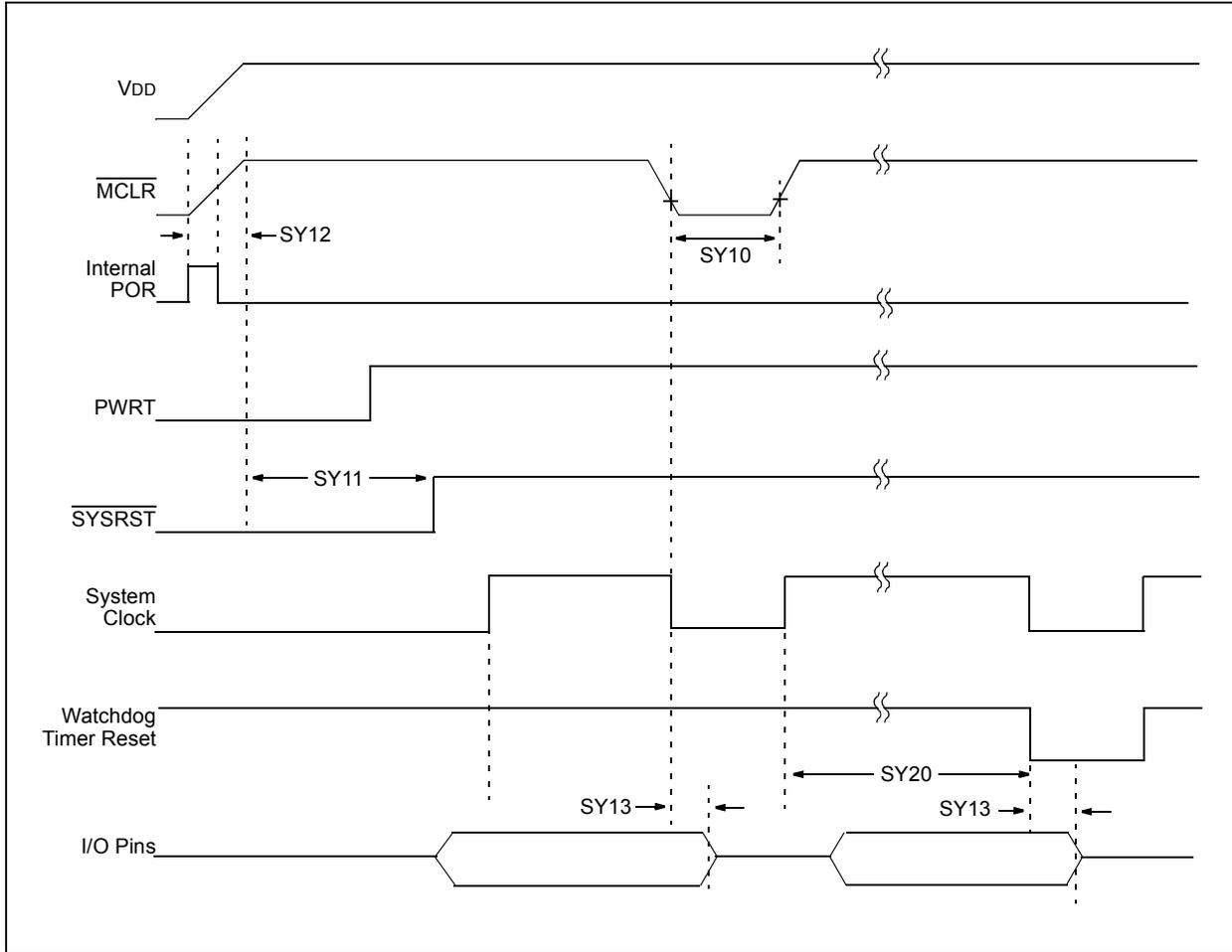
**TABLE 28-21: RESET, WATCHDOG TIMER, OSCILLATOR START-UP TIMER, POWER-UP TIMER AND BROWN-OUT RESET TIMING REQUIREMENTS**
