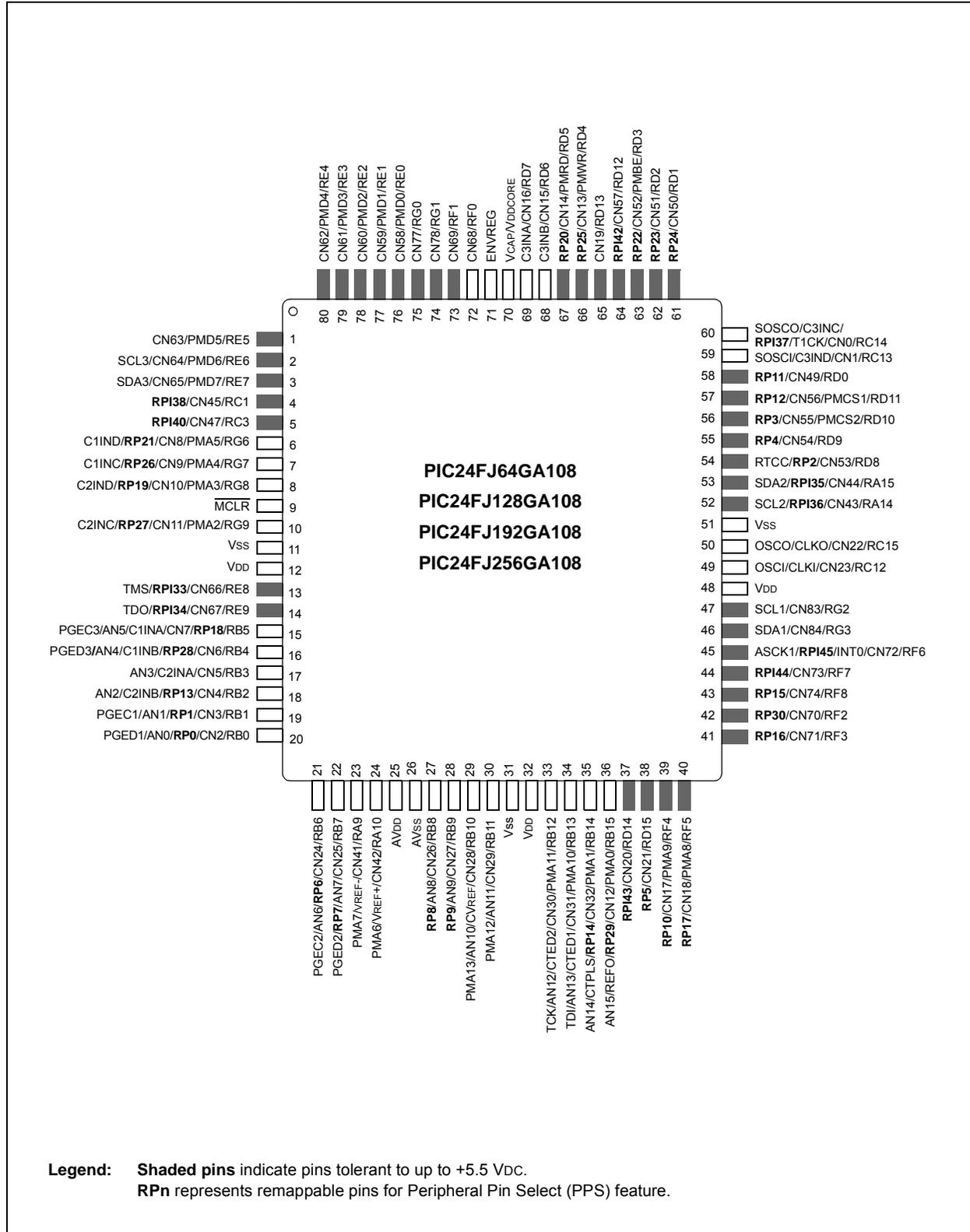
**Legend:** Shaded pins indicate pins tolerant to up to +5.5 Vdc.
