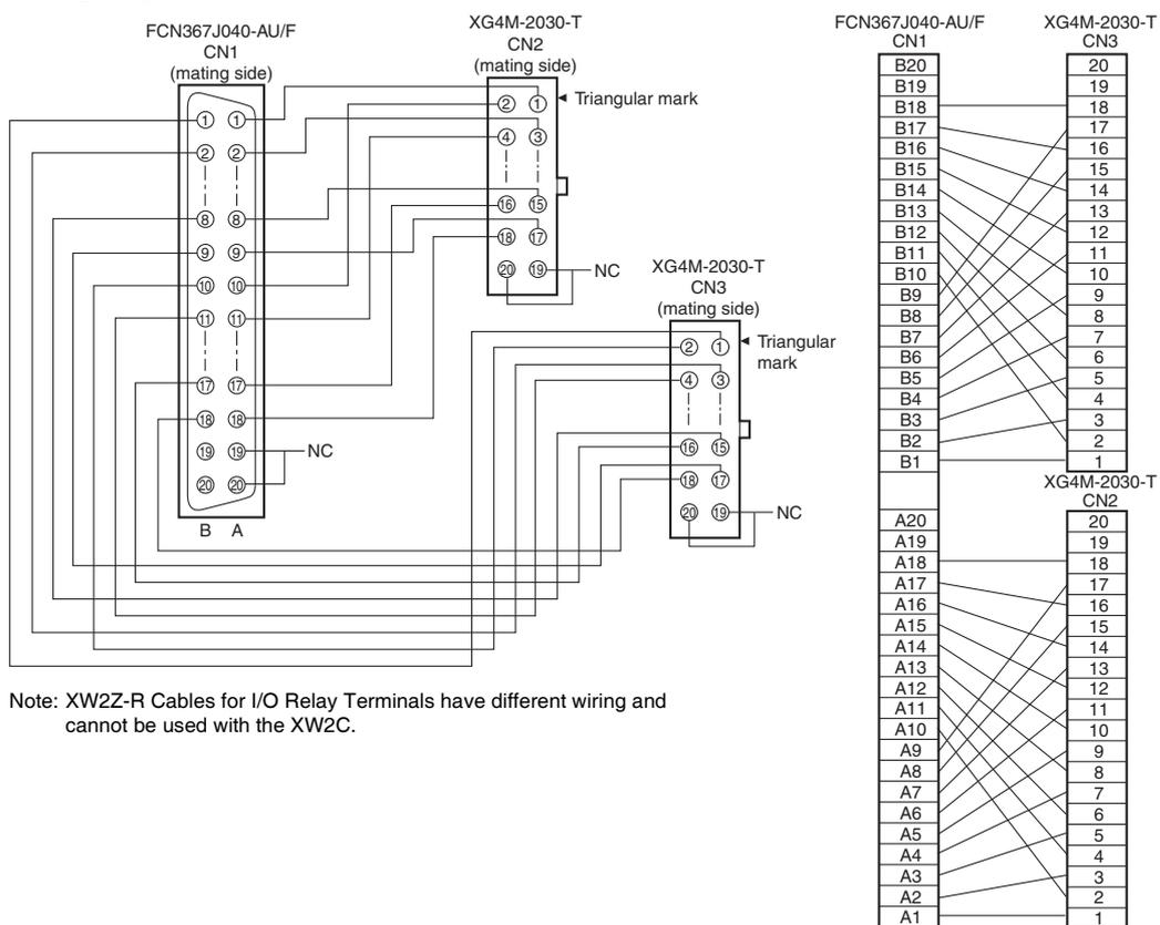
**20-pole Cable with Discrete-wire Press-fit Terminals**
