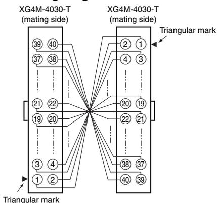
Note: Connector pins are connected 1-to-1 so that pin numbers correspond.
