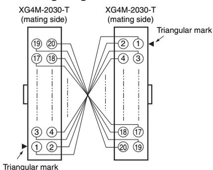
Note: Connector pins are connected 1-to-1 so that pin numbers correspond.
