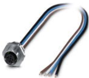
Flush-type connector, Universal, 4-position, Socket, M12, A-coded, Front mounting, M16 x 1.5, Individual wires, cable length: 0.5 m
