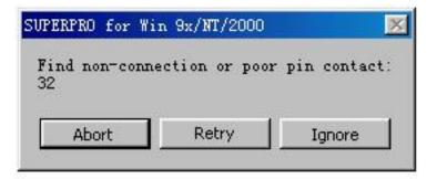
In the case of the diagram above, for example, pin 32 has trouble. The resolution is:
