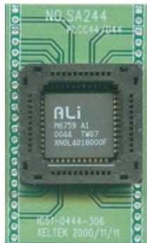
•Adapters are inserted in the same way as DIP devices.
