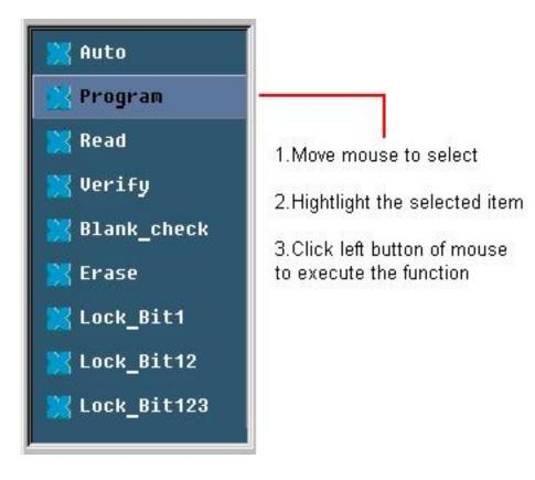
The function displayed may differ from chip to chip. The frequently-used operations are explained below.
