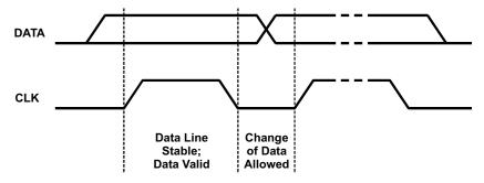
Figure 31. Bit Transfer on the Serial Interface
