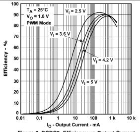
Figure 8. DCDC2: Efficiency vs Output Current
