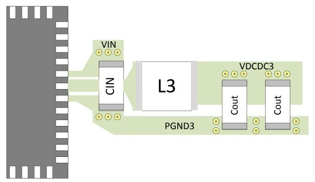
Figure 45. Layout Example of a DC-DC Converter
