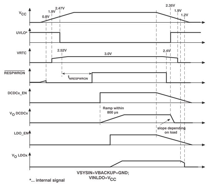
Figure 2. Power-Up and Power-Down Timing
