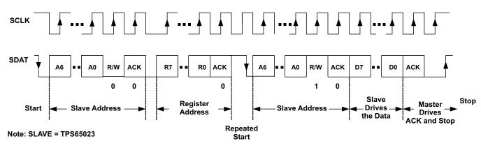
Figure 34. Serial I/F READ from TPS65023x: Protocol A
