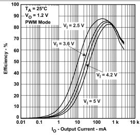
Figure 6. DCDC1: Efficiency vs Output Current
