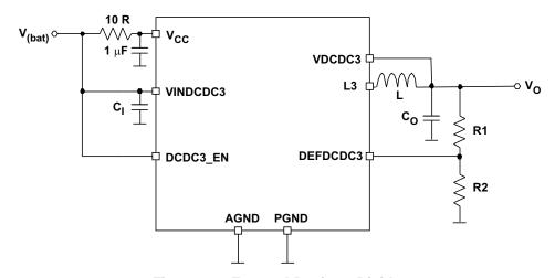
Figure 41. External Resistor Divider
