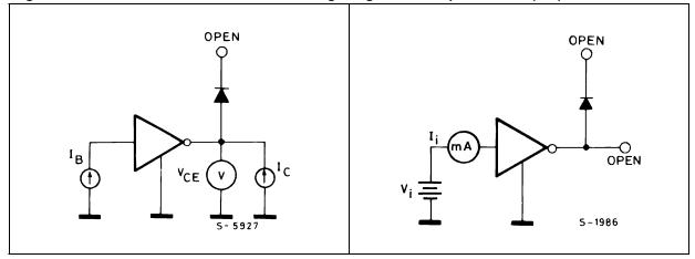
Figure 7. Input voltage Figure 8. Clamp diode leakage current OPEN V<sub>CE</sub> S - 5727 S - 1987
