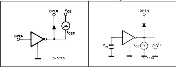
Figure 5. Collector-emitter saturation voltage Figure 6. Input current (ON)
