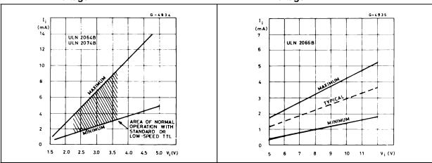
Figure 13. Collector current as a function of input current
