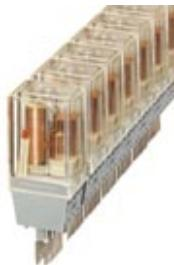
Relay connector, equipped with Hengstler miniature round relay, contacts (AgCdO+Au): small to large loads, 2 PDT, input voltage 24 V AC, with light indicator, can be plugged on basic termination blocks
