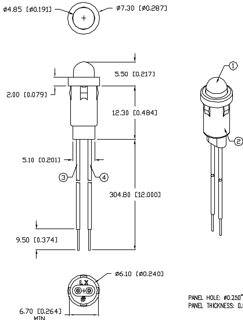
\*UNLESS OTHERWISE SPECIFIED TOLERANCES PER DECIMAL PRECISION ARE: X=±1 (±0.039), XX=±0.5 (±0.020), XXX=±0.25 (±0.010), XXXX=±0.127 (±0.005). LEAD SIZE=±0.05 (±0.002), LEAD LENGTH=±0.75 (±0.030). MIN= <sup>+0.00</sup><sub>-0.00</sub> DECIMAL PRECISION MAX= <sup>+0.00</sup><sub>-0.00</sub> DECIMAL PRECISION
