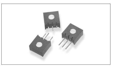
These long established 10mm square, single turn potentiometers will meet a wide range of industrial and professional applications. Cermet element technology ensures stability and reliability. This P.C.B. mounted package has easy top or side adjustment, or finger adjust styles. All components are sealed to withstand printed circuit board washing solvents.
