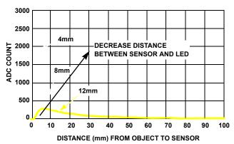
12-BIT ADC, 4k GAIN, 12.5mA LED NO LIGHTPIPE, NO FILTER/GLASS. NO BARRIER 18% KODAK GRAY CARD AS REFLECTOR
