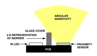
FIGURE 18. DIAGRAM OF PROXIMITY SET-UP
