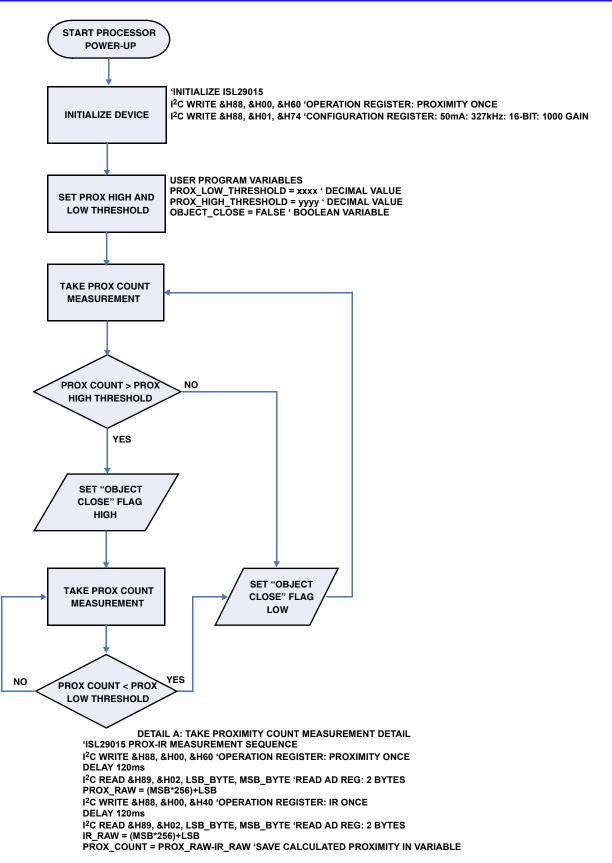
FIGURE 22. FLOW-CHART FOR PROXIMITY SYSTEM DETECTING HUMAN SKIN
