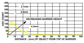
12-BIT ADC. 4k GAIN. 12.5mA LED LED ENCIRCLED BY BARRIER NO LIGHTPIPE 4mm CENTER-TO-CENTER LED TO SENSOR 18% KODAK GRAY CARD AS REFLECTOR
