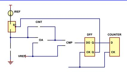
FIGURE 2. 16-BIT CHARGE INTEGRATION ADC
