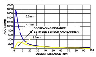
12-BIT ADC. 4k GAIN. 12.5mA LED LED ENCIRCLED BY BARRIER 2.1mm NO LIGHTPIPE, NO FILTER/GLASS 4mm CENTER-TO-CENTER LED TO SENSOR 18% KODAK GRAY CARD AS REFLECTOR
