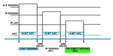
FIGURE 3. INTEGRATION TIMING SEQUENCE FOR PROXIMITY DETECTION
