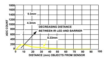
12-BIT ADC. 4k GAIN. 12.5mA LED SENSOR ENCIRCLED BY BARRIER 2.1mm NO LIGHTPIPE, NO FILTER/GLASS 4mm CENTER-TO-CENTER LED TO SENSOR 18% KODAK GRAY CARD AS REFLECTOR
