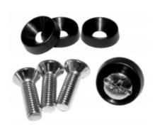
The 1421A screw provides a standard 0.625" rack screws length with 10-32 threads. The screw itself features a slotted and phillips, oval head and has a nickel plate finish. The black plastic cup washers have an outside diameter of 0.58".
