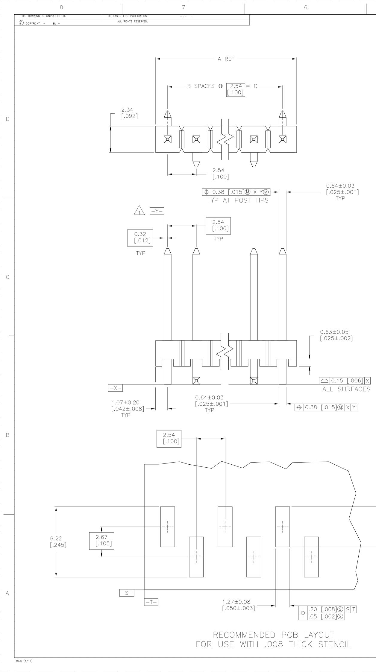
THE NOTED DIMENSIONS APPLY AT THE INTERSECTION OF THE POST AND THE HOUSING 0.000762[.000030] GOLD ON CONTACT AREA, 0.00254[.000100]-0.00508[.000200] MATTE TIN-LEAD ON SOLDER TAIL, ALL OVER 0.00127[.000050] NICKEL.
