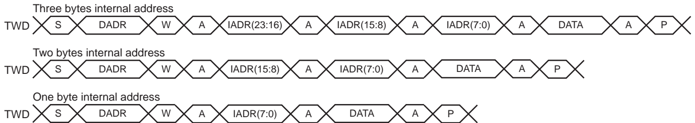
Figure 40-10: Master Write with One, Two or Three Bytes Internal Address and One Data Byte
