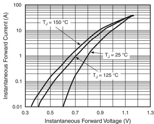
Fig. 3 - Typical Forward Characteristics Per Diode
