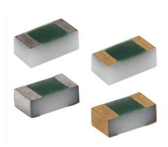
FC series chip resistors are designed with low internal reactance. They function as almost pure resistors on a very high range of frequencies. The specialized laser edge trimming allows for precision tolerances to 0.1 %.
