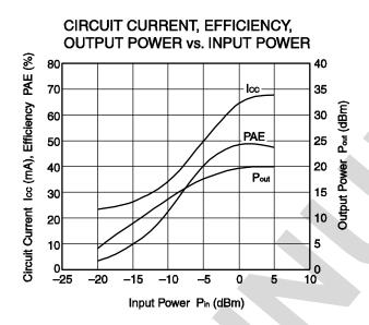
Condition: f = 2 450 MHz, Vcc1 = Vcc2 = Vbias + Venable = 3.0 V, Pin = 0 dBm, with external input and output matching circuit
