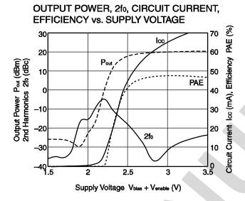
Condition :  $Vcc1 = Vcc2 = V_{bias} + V_{enable} = V_{cont} = 3.0 \text{ V}$ ,  $P_{in} = -20 \text{ dBm}$ , with external input and output matching circuit
