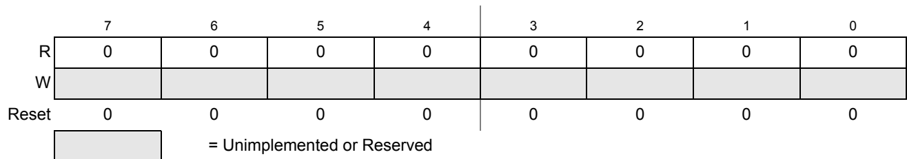
Figure 28-8. Flash Reserved0 Register (FRSV0)
