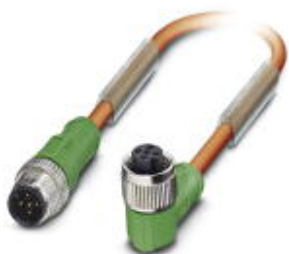
Sensor/actuator cable, 5-position, PUR, orange RAL 2003, Plug straight M12, A-coded, on Socket angled M12, A-coded, cable length: 1 m, Customer-specific version
