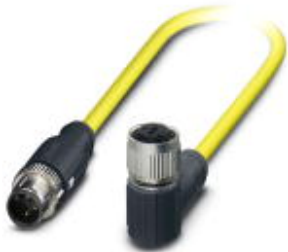
Sensor/actuator cable, 3-position, PVC, yellow, shielded, Plug straight M12 SPEEDCON, coding: A, on Socket angled M12 SPEEDCON, coding: A, cable length: 1.5 m
