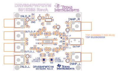
Figure 16. DRV604PWPEVM PCB Component Placement
