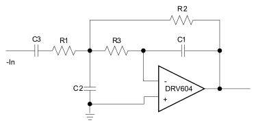
Figure 3. 2<sup>nd</sup> Order Active Low-Pass Filter, SE Input
