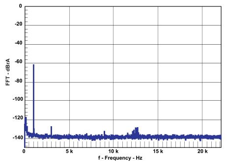
Figure 9. FFT Spectrum with -60-dBFS Tone (Head-Phone Output)
