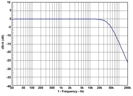
1Vrms output,  $10k\Omega$  load, 500kHz measurement filter, 2Vrms reference
