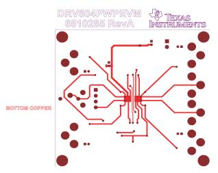
Figure 18. DRV604PWPEVM PCB Bottom Layer
