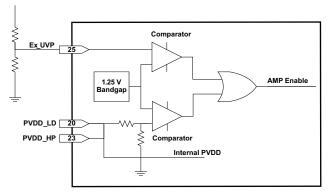
The external under voltage detection can be used to shutdown the DRV604 before an input device can make a pop. The shutdown threshold at the UVP pin is 1.25V. A resistor divider is used to obtain the shutdown threshold and hysteresis desired for the application.
