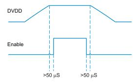
Figure 2. Power-Up/-Down Sequence
