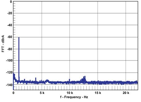
Figure 8. FFT Spectrum with -60-dBFS Tone (Line Output)
