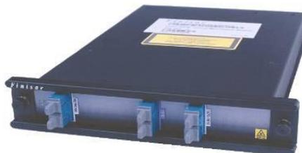
1550/CWDM plug-in module is a passive optical multiplexer /demultiplexer designed to add CWDM wavelengths to an existing 1550nm backbone ring. The module multiplexes and demultiplexes a single 1550nm wavelength and the complete CWDM wavelength grid from a two-fiber ring network.
