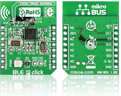
BLE P click™ is a simple solution for adding a Bluetooth 4.0 (alternatively known as Bluetooth Low Energy) peripheral device to your design. It communicates with the target board through **mikroBUS™** SPI (CS, SCK, MISO, MOSI), INT (RDY) and AN (ACT) lines. Beside the mikroBUS™ socket, BLE P click™ also features additional UART input and output pins (RXD and TXD). These enable you to test the RF parameters of the BLE P's radio design. The board uses a 3.3V power supply only.
