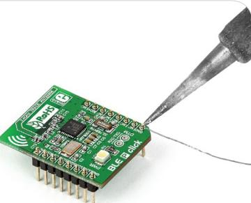
Turn the board upward again. Make sure to align the headers so that they are perpendicular to the board, then solder the pins carefully.
