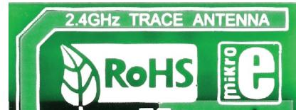
BLE P click™ features a PCB trace antenna, designed for the 2400-2483.5 MHz frequency band. Maximum device range is up to 40 meters in open space.
